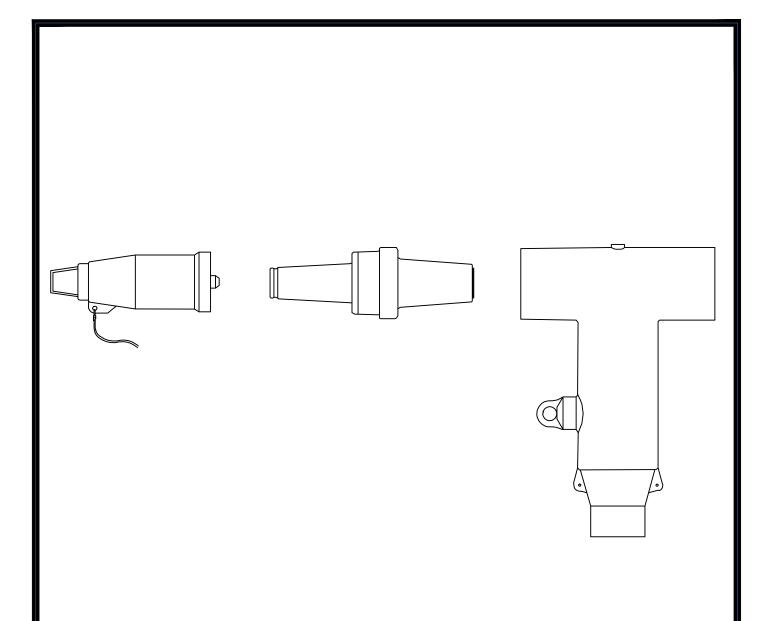
Note: All "T" Connector kits come with a tap plug reducer with stud and pro cap as shown above.
